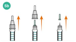
Pull off the outer needle cap and save it.
