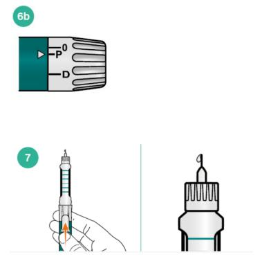
Hold the Kauliv pen with the needle pointing up. Push and hold the release button towards the needle until the arrow on the dose selector points to **0**. Keep dialling to **P** and releasing until a drop of teriparatide appears at the needle tip (fig. 7). The Kauliv pen is now ready for use. (If the arrow does not return to **0** after pushing the release button, refer to the priming advice given above.)
