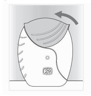
Slide the cover upwards as far as it will go, to cover the mouthpiece.
