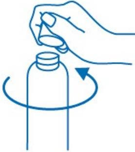
Mounting the dosing pump on the bottle:
