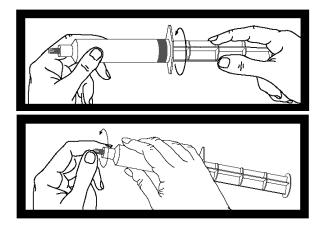
After screwing the push rod into the syringe piston, it is important to **turn the push rod an additional** <sup>1</sup>/<sub>2</sub> **turn** so that the grey piston rotates freely
