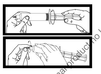
After screwing the push rod into the syringe piston it is important to **turn the push rod an additional** <sup>1</sup>/<sub>2</sub> **turn** so that the grey piston rotates freely.
