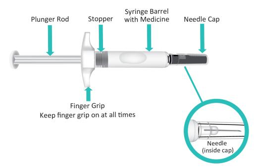
Figure A: TAKHZYRO pre-filled syringe
