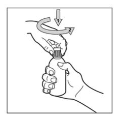
Step 3. Insert the bottle adapter in the bottle neck opening. You may need to apply some pressure to insert it securely. Once inserted, the bottle adapter must not be removed from the bottle. The bottle can be closed with the closure with the bottle adapter still in place.
