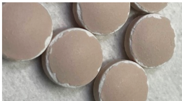
Figure 8: Example of erosion and film cracking of a \text{CaO}_3 film coated tablets
