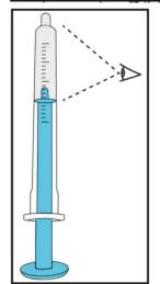
d. Carefully check for air in the blue syringe. Smaller air bubbles are not critical.
