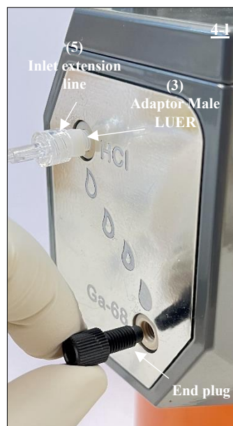
Fig. 21 Removing the end plug from the Ga-68 port of the radionuclide generator.
