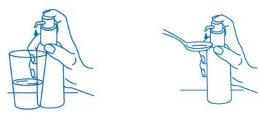
The dosing pump head can then be released and is ready for the next pump actuation.
