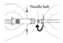
To attach the needle, connect the hub to the Luer Lock Adaptor and rotate a quarter turn clockwise until you feel it lock.
