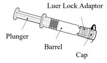
Hold the syringe by the barrel, not by the plunger. Unscrew the syringe cap by twisting it anticlockwise.
