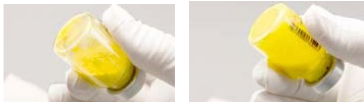
Unsuspended: visible clumps Suspended: no clumps Figure B: Check for unsuspended powder and repeat tapping if needed.
