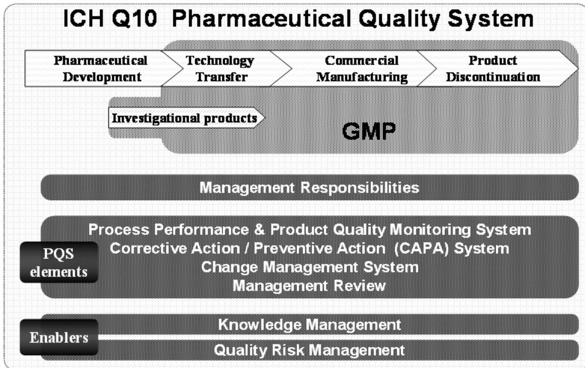
This diagram illustrates the major features of the ICH Q10 Pharmaceutical Quality System (PQS) model. The PQS covers the entire lifecycle of a product including pharmaceutical development, technology transfer, commercial manufacturing, and product discontinuation as illustrated by the upper portion of the diagram. The PQS augments regional GMPs as illustrated in the diagram. The diagram also illustrates that regional GMPs apply to the manufacture of investigational products.
