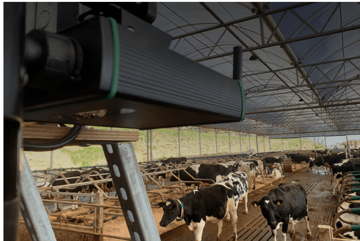
HerdVision 3D camera mounted above race to monitor BCS & mobility.
