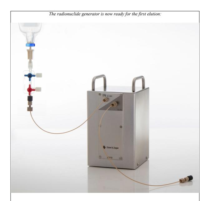
Please note: The radionuclide generator is designed not to drain itself, when no lines are connected to the inlet and outlet ports, but it is <u>not recommended</u> to leave the ports open at any time. When the container with the sterile ultrapure 0.1 mol/l hydrochloric acid is connected and the fluid path is open, the radionuclide generator will be eluted by gravity. Therefore, it is necessary to keep the inlet and outlet lines as well as the positions of the stopcock valves under control.
